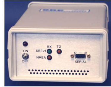
90488 SEACAT/SEALOGGER RS-232 & Navigation Interface Box
