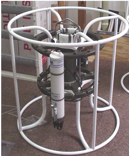
SBE 32C shipped fully assembled (Note: CTD shown in photo is not included with standard shipment)
