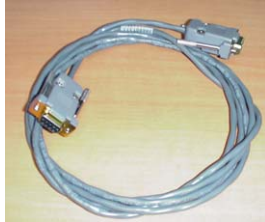
171887 Computer to Deck Unit cable for Serial Data & Carousel Data connectors (2 cables / SBE 33)
