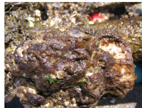
SBE 43 after 4 months in Shilshole Bay (see data on next page, far right)
