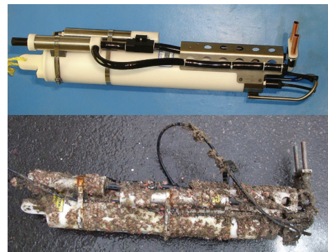
SBE 16plus with SBE 43 before and after 5 months in Cockburn Sound -- note, intake and exhaust protected from biofouling by copper extensions
