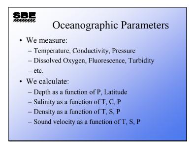
We measure physical quantities with Sea-Bird instruments. These quantities are then used to calculate the many parameters that are found in the analysis of oceanographic data. Because the calculated parameters rely on accurate measurement of the physical quantities, a small error in the original measurement can result in a large error in data analysis.
