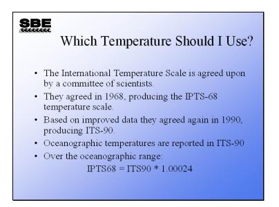
The calculation of the parameters mentioned on the previous slide is made with equations of the physical parameters. These equations were derived by gathering data in a laboratory relating T, P, and C to the parameter of interest, and statistically fitting the data to high order polynomials. The coefficients of the polynomials were determined using the 1968 temperature scale. So, to use these high-order polynomials, we must convert to the 1968 temperature scale for these calculations.
