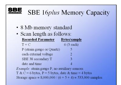
The SBE 16*plus* has considerably more memory than the 16, with 8 Mbytes of non-volatile flash memory. Again, memory capacity depends on the configuration of the instrument.
