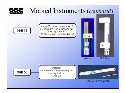
The SBE 39 is a temperature recorder, and may also be equipped with a pressure sensor. An example of its use is mounted on bottom trawls to measure bottom depth, time on bottom, and temperature. The SBE 39 is available with RS-232 serial interface or inductive modem interface (39-IM). The SBE 39 and 39-IM have a 600-meter plastic or 10,500-meter titanium housing.
