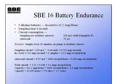
Recall the slide on memory endurance for the SBE 16. We can calculate that we have memory for 115,918 samples if measuring temperature, conductivity, and Digiquartz pressure, with no auxiliary sensors (115,918 = [1,048,576 - 5308] / [4 + 5]). This is enough memory for 19,319 hours of operation if sampling every 10 minutes. We will run out of battery power before we run out of memory.
