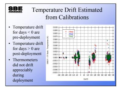
JAMSTEC has installed calibration equipment, nearly identical to Sea-Bird's equipment, that allows them to monitor the drift of their sensors before they are deployed. The plot above shows drift of their temperature sensors before and after deployment at three temperatures. As you can see from the plot, with a few exceptions the thermometers are very stable:  $\pm 0.002$  °C is within the initial accuracy specified for the SBE 37.
