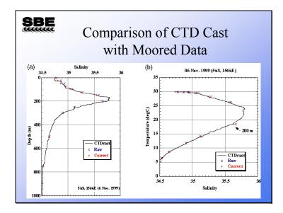
Here is a plot of a CTD cast with the mooring data overplotted on it. Raw and corrected values are shown. Although the scale is rather coarse, the correction improved the agreement between the instruments.
