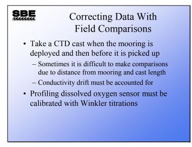
Sea-Bird does not supply software to correct time series data. These corrections are similar to those done on a cast basis for profiled data. An incremental offset is applied to temperature data, assuming the offset drift is linear and monotonic throughout the deployment. For conductivity, an incremental slope is applied to the time series, again assuming that the slope change is linear and monotonic throughout the deployment period.
