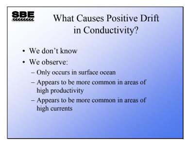
We have no substantiated ideas regarding positive drift, although it has been observed by researchers in various parts of the world. Anecdotally, when positive drift is observed, it occurs in the instruments in the surface part of the mooring. Also, it seems to occur in areas of high productivity and in areas with strong surface currents.
