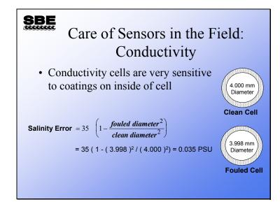
Conductivity sensors are another matter. Recall this slide from a previous discussion. A very thin coating can change the cell geometry, having a large effect on the conductivity measurement.
