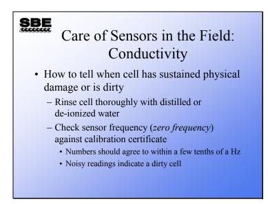
As we discussed in another module, checking the zero frequency of a conductivity cell is a great way to do a spot check on the health of the sensor.
