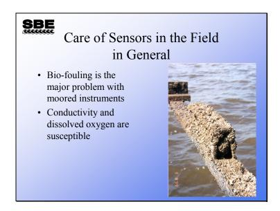
This SBE 37 is deployed in the tide waters of Georgia. Biological activity surges when the water temperature exceeds 20 °C. The researcher uses extra bio-fouling protection on each end of the conductivity cell and protects the pressure housing of the instrument with packing tape and silicon grease.
