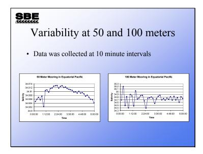
We are going to be comparing data collected by moored instruments with data collected in a CTD profile. It is important to keep in mind that even though the mooring is fixed in place, the ocean moves around it. There can be substantial variability over a fairly small time interval. Most of the time there is little hope of having the CTD in place at the moment the moored instrument is taking a measurement.
