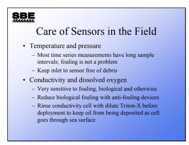
As we have discussed, thermometers are very robust. In moored applications, the sampling interval is much longer than the time constant of the thermometer, so except in extreme conditions fouling does not affect thermometers.
