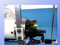
Align the dimple on the connector boot with the large pin on the connector. Remember to *burp* the connector(s) after installation.
