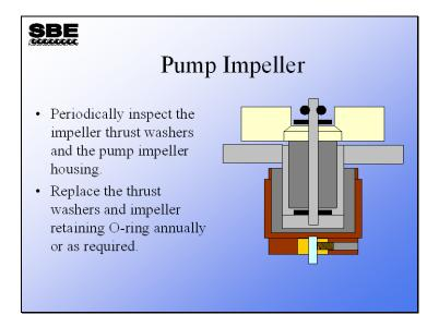
There is a grove for the impeller retaining O-ring in the tip of the shaft. Push down with your fingertip until the ring slips into the groove.
