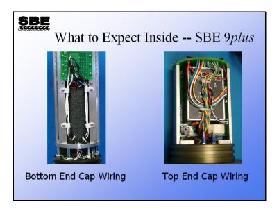
Note that the wiring from all of the connectors joins together to form large bundles.
