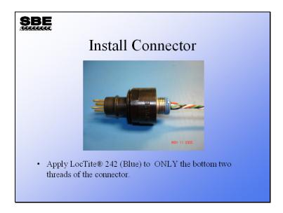
You should stop seeing LocTite® move up the threads when there are approximately two full threads remaining on the connector.
