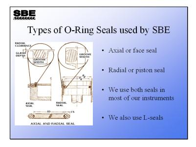
The face seal and piston seal are used in conjunction with each other on the battery end cap.
