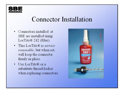
If you use a substitute thread-locker, make sure that it indicates that it is *service* removable and is rated for  $\frac{1}{2}$ " hardware.
