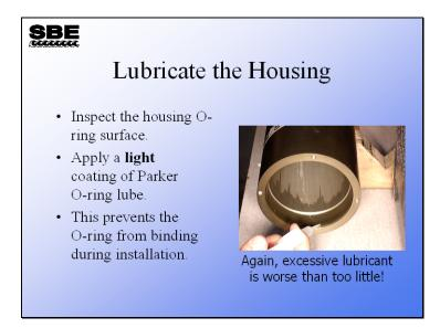
Inspect for pits, scratches, corrosion, and foreign matter.
