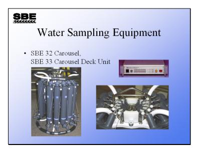
As a companion to CTD profilers, Sea-Bird supplies water sampling equipment. Sea-Bird manufactures the framework, mechanism for closing bottles, and deck power supply and sampler control. The water sample bottles themselves are not manufactured by Sea-Bird. The SBE 32 is the portion of the equipment that triggers the bottle closure.
