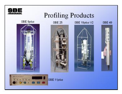
Sea-Bird offers 4 profiling instruments: the real-time SBE 9*plus*/11*plus* system, the internally recording SBE 25 and SBE 19*plus* V2, and the real-time SBE 49. The capabilities of these instruments are contrasted in the following pages.
