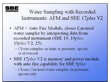
Internally recording instruments output a real-time, RS-232 serial data stream. This data stream is suitable for real-time telemetry over short cables only. The data stream is used by the AFM to monitor the depth of the sampling package for the purpose of closing water samplers.
