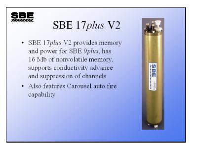
The SBE 17*plus* V2 acts as battery power and internally recording memory for the SBE 9*plus*. This device has the capability to close water samplers as well. It only closes bottles on the upcast.
