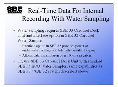
The SBE 19, 19*plus*, 19*plus* V2, and 25 can be equipped with water sampling equipment. The SBE 33 Carousel Deck Unit and SBE 32 Carousel (or SBE 55 ECO) provides power and telemetry for the CTD very similar to the 11*plus / 9plus* setup. In addition to water sampling, this equipment allows data telemetry over 10 km of sea cable and supplies more than enough power for the CTD and auxiliary sensors.
