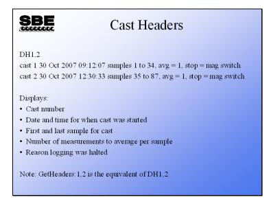
Each cast header lists the start date and time, number of scans in the cast, number of samples averaged per scan, and reason the cast ended for each cast.
