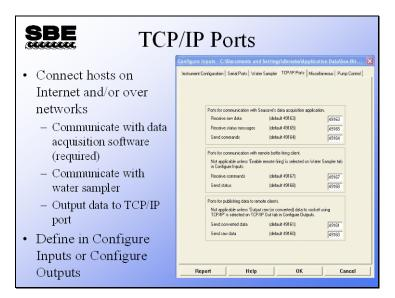
TCP/IP (Transmission Control Protocol / Internet Protocol) is a set of communications protocols used for the Internet and other similar networks. Transmission of Seasave data via TCP/IP allows you to view real-time data and to fire water sampler bottles at a remote computer on the ship.
