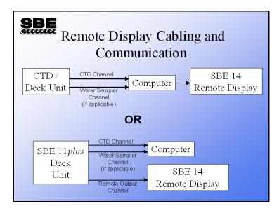
The SBE 14 remote display can be cabled to your system in one of two ways:
