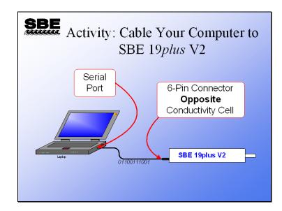
The 6-pin Data I/O - Pump connector is 180° from the conductivity cell. In class, we are connecting to this with a 6-pin to 4-pin adapter cable and a 4-pin to DB-9 data I/O cable. [The other connectors are for auxiliary voltage sensors (three 6-pin connectors) and an auxiliary RS-232 sensor (one 4-pin connector).]
