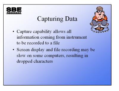
The capture capability allows Seaterm232 to place all characters received into a file. This is useful for testing instruments, performing diagnostics, or in some cases recording realtime data. Note that there is no testing of data integrity and the act of displaying the characters on the screen while they are being written to a file may cause some characters to be lost.
