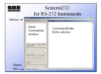
Seaterm232 opens if you select *SBE 19plus V2* in SeatermV2's Instruments menu. Seaterm232 is compatible with instruments with an RS-232 interface: 16*plus* V2, 19*plus* V2, 37(-SM, SMP, SI, SIP), and SBE 54. Seaterm485 and SeatermIM have similar menus and functions.
