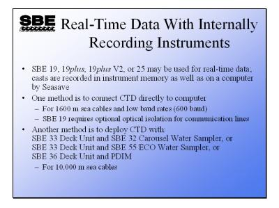
SBE 19s may be outfitted with high power cable drivers and optical isolation for transmitting real-time data. The SBE 19*plus*, 19*plus* V2, and 25 come standard with this equipment. With the addition of a Deck Unit and associated underwater equipment listed above, the data telemetry is the same as discussed for the SBE 911*plus*.
