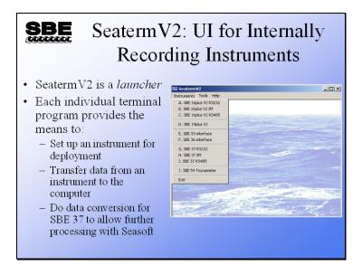
SeatermV2 is a terminal program *launcher* intended for use with Sea-Bird instruments developed or redesigned in 2006 and later. The common feature of this generation of instruments is the ability to output data in XML. SeatermV2 launches one of the following terminal programs, depending on the communication protocol required:
