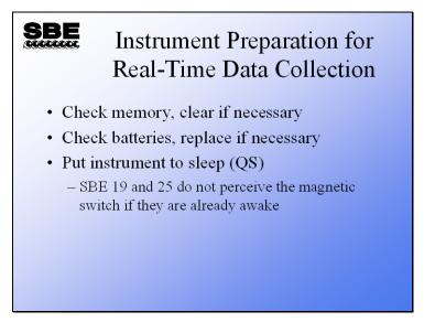
Unlike the SBE 19 and 25, the SBE 19*plus* and 19*plus* V2 **do not** have to be asleep when you move the magnetic switch to the On position.
