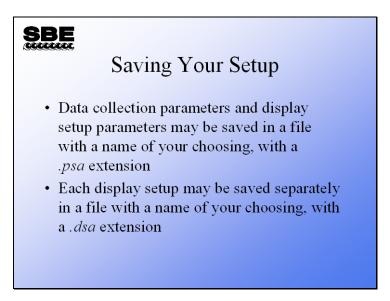
Setup files are handy for different instrument types or for pre-deployment instrument checkout *vs*. deployment display. For example, you might use fixed display or scrolled display for pre-deployment check out and then switch to a full screen plot for the cast.
