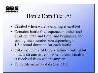
Whenever a bottle confirmation is received by Seasave from either the confirm status bit or via the modem port, a line is written to the output file with a .bl extension. This contains the bottle firing sequence number, bottle position, date, time, and beginning and ending scan number for the fired bottle. It is used in data processing to build up a larger file of data parameters collected while the water sampler was being closed.
