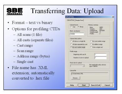
When you click the Upload menu in Seaterm232, you start a process that produces an upload file that is compatible with our data processing software (SBE Data Processing).
