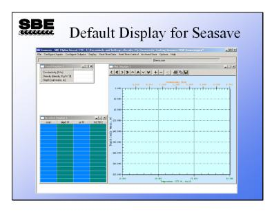
The slide above has all three data windows visible. The top left window is a fixed display and the bottom left window is a scrolling display. The right window is a multi-axis plot.
