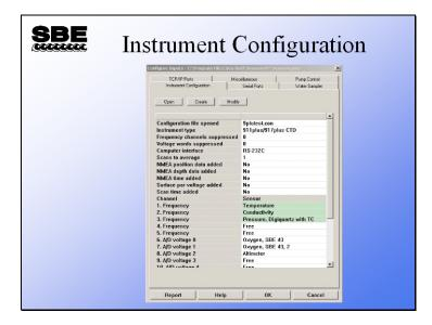
Click the Configure Inputs menu to get the Configure Inputs dialog box; the first tab is the Instrument Configuration tab. From the Instrument Configuration tab, you can open and examine an existing .con or .xmlcon file, or create a new .con or .xmlcon file.
