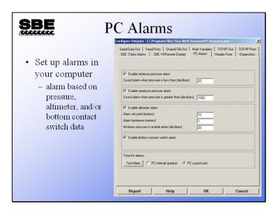
You can also set up an audible alarm in your computer that may be triggered by minimum pressure, maximum pressure, altimeter data, and/or bottom contact switch data.
