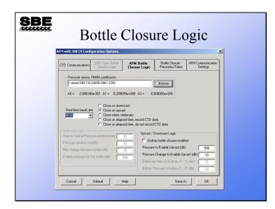
The bottle closure logic tab contains almost all the information that the AFM, SBE 17*plus* V2, or SBE 55 ECO need to close water sample bottles based on the closure protocol you select.
