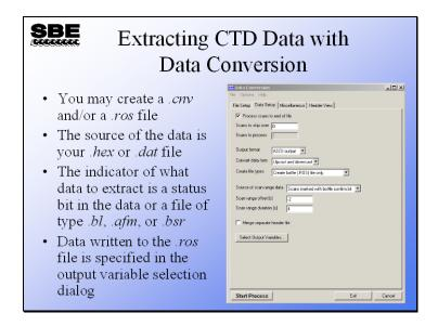
The Data Conversion module creates a .ros file containing the same variables that the .cnv file contains, with scans logged around the moment a water sample was collected. For real-time water sampling, Data Conversion determines when the water sample was taken by:
