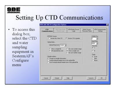
The CTD communications form allows you to select the communications parameters for your instrument as well as data transfer protocol and header options. Instruments with older firmware revisions are not able to change baud rate during data transfers.
