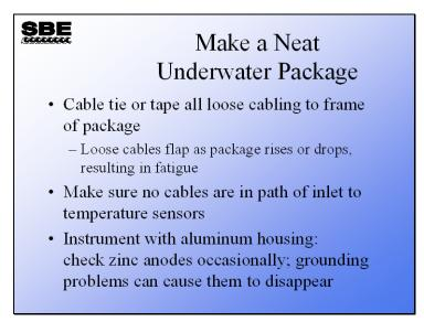
Neatness counts! Secure all your loose cables. When you lower your instrument package at 1 meter per second, any loose cabling will flap. This sort of repetitive motion will fatigue the cables and shorten their working life.
