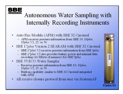
Sea-Bird offers several products for closing water sampler bottles remotely. These products receive pressures from the CTD and are programmed to close bottles on operator-chosen criteria.
