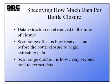
The range of data to copy out of the .cnv file into the .ros file is specified in seconds. You may copy a maximum of 1440 scans per bottle closure. For an SBE 9*plus* system operating at 24 Hz, 4 seconds of data is 96 scans. For an SBE 19 operating at 2 Hz, 4 seconds of data is only 8 scans.
