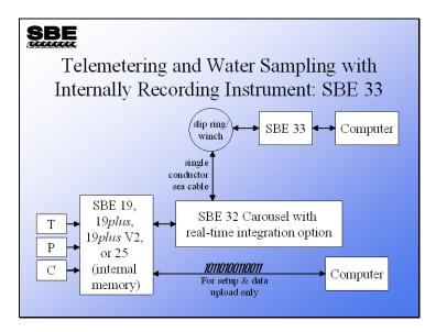
This setup can also be used with an SBE 49 FastCAT CTD, which has no internal memory.
