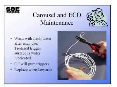
The trigger mechanism of the Carousel and the ECO is made of titanium. The titanium pieces are coated with Tiodizing; this product is similar to anodizing aluminum. The Tiodized surface is water lubricating and should **never** be oiled with petroleum or silicon-based products. Rinse your trigger mechanism with fresh water after each cast and clean it periodically with soap and water.
