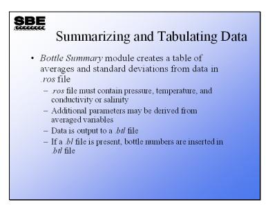
The *.ros* file created by *Data Conversion* contains a set of data scans for each water sample taken. The *Bottle Summary* module takes the process one step further by averaging the scans for each water sample into a single line of data that contains averages and standard deviations for each of the parameters in the *.ros* file. In addition, you may add derived parameters to this list. The derived parameters are calculated from the averages of the data contained in the *.ros* file.
