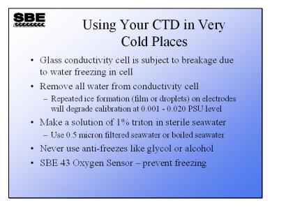
Another option in place of a Triton solution for the conductivity cell is the use of a brine solution (distilled seawater or homemade salt solution that is higher than 35 psu in salinity), as salty water depresses the freezing point. However, there is still a risk of forming ice inside the conductivity cell if deploying through frazil ice on the surface, if the freezing point of the salt water is the same as the water temperature.
