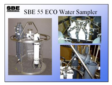
The SBE 55 is a small, 3- or 6-bottle water sampler, intended for sampling in depths to 600 meters. Its trigger mechanism operates in the same way as the mechanism on the Carousel, and its electronics are similar.
