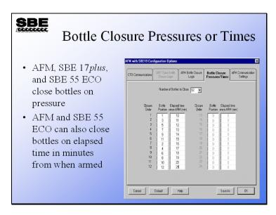
Once you have defined the governing bottle closure logic – on upcast, on downcast, when stationary, or on elapsed time – you need to enter the number of bottles to close and which bottle to close when. Bottles may be closed in any order desired.
