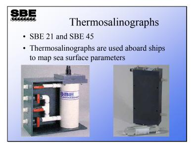
Thermosalinographs are used to collect information about the sea surface; typically in flow-through systems operating continuously throughout a cruise. They are included in the profiling section of the course because they are installed on many research vessels. Thermosalinographs are typically installed inside and near to the hull of a ship in order to make measurements on uncontaminated seawater. Optionally, you can plumb other types of sensors into the system for a wider range of measurements.
