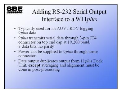
As an option, an RS-232 Serial Output interface can be installed in the *9plus*, in place of the interface for the G.O. 1015 Rosette.
