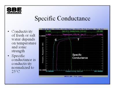
The conductivity of fresh or salt water is strongly dependent on temperature, as shown above by the similarity in the shape of the C and T plots. Specific conductance is typically used for fresh water applications, where the salinity equation is out-of-range. It allows us to visualize the conductivity without the temperature dependence, providing some indication of the amount of salts in the water.
