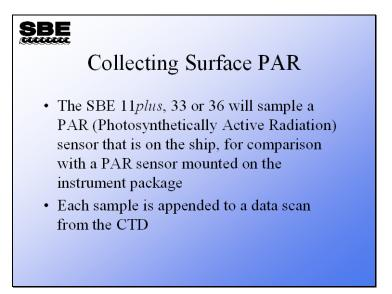
Sea-Bird deck units may be equipped with an A/D interface intended to digitize the signal from a deck-mounted PAR sensor. This is standard equipment for the SBE 11*plus* and optional for the SBE 33 and 36. In Seasave, Surface PAR data is appended to real-time data if you select *Surface PAR voltage added* in the instrument configuration (*.con* or *.xmlcon*) file dialog box.
