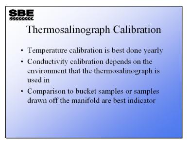
These are recommendations only; the conductivity calibration depends on the environment that the thermosalinograph is operated in.
