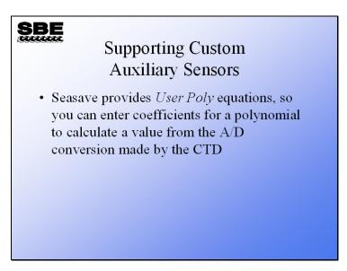
For instruments that are not supported in Seasave, a meaningful display of data can be made by specifying a *user polynomial* to be applied to the 0 - 5V data. The user polynomial can be up to  $3^{rd}$  order:
