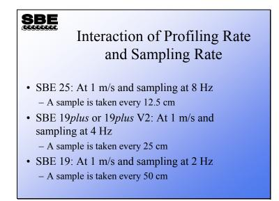
As discussed earlier, the lower sample rates of the SBE 19, 19*plus*, 19*plus* V2, and 25 translates into a coarser resolution than that calculated in the SBE 9*plus* example. The following page illustrates the impact that sample rate has on resolution.
