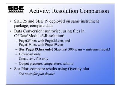
After running SBE Data Processing's Data Conversion module, we should end up with the following files, which we will plot in Sea Plot to see the effect of sampling rate on the resolution:
