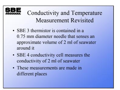
The active part of the thermometer is found at the end of the slender needle. The volume of water measured by the end of the needle is approximately 2 ml.
