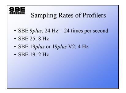
Sea-Bird offers CTDs with sampling rates shown above. The SBE *9plus*, with the fastest sampling rate, produces the most detailed data. The other instruments are less capable but offer lower price, less complex deployment equipment, and a more compact instrument package. Not all applications require or benefit from the sampling rates achievable with the SBE *9plus*.
