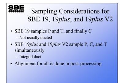
The SBE 19 has a different sampling protocol than the SBE 25 and the *9plus*. The 19 uses the same signal condition circuit, an oscillator, to sample both T and C. A relay switches the oscillator between the thermistor and the conductivity cell. Further, to improve circuit stability, reference resistors are switched into the oscillator every 120 samples.
