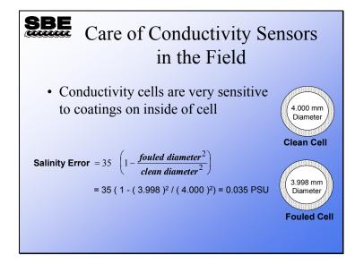
Conductivity sensors have parts that interact with the seawater. There are 3 electrodes that are subject to fouling, and a cell that must maintain constant dimensions. As the slide shows, a 0.001 mm coating will diminish the cell diameter by 0.002 mm, resulting in a salinity error of 0.035 PSU. A film thickness of 0.001 is not uncommon for oils on the sea surface. Another source of fouling is bacterial colonization.
