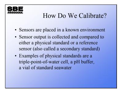
To calibrate a sensor, it is placed in a precisely controlled environment. The output of the sensor is collected at the same time as the environment is measured with a reference sensor. The reference sensor is carefully calibrated and has a well-known history. To gain the careful calibration and history, the reference is calibrated against physical standards such as the triple point of water and the melting point of gallium, or an agreed-upon standard such as IAPSO standard seawater.
