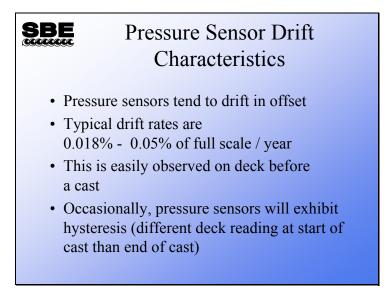
Pressure sensors are usually trouble-free. Drifts are generally in offset. The drift may be read on deck and entered into the coefficient dialog box to make the correction.
