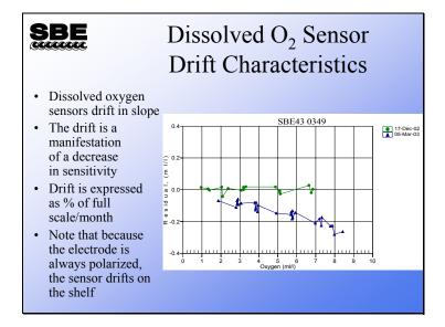
Dissolved oxygen sensor drift, like conductivity sensor drift, can be episodic in nature. It also has similar causes. The sensor depends on the diffusion of oxygen through a Teflon membrane. Any surface coating that slows the diffusion will affect the sensor sensitivity and its time response.
