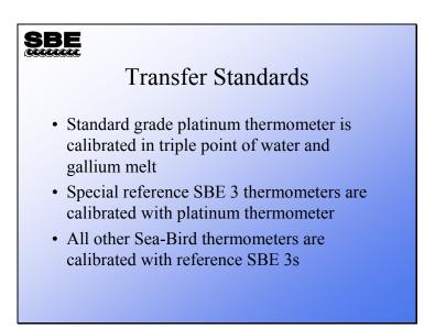
As was previously mentioned, a platinum thermometer is calibrated in the fixed point cells and then used to calibrate the SBE 3 reference thermometers. The platinum thermometer is susceptible to calibration shift due to impact or vibration; because of this it is impractical to use it in routine calibration. The SBE 3s are much more robust. By careful selection of the SBE 3 and the accumulation of a drift history, very accurate calibrations can be accomplished.
