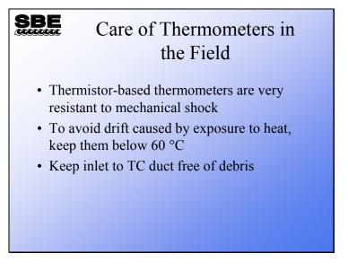
SBE 3 thermometers are essentially trouble-free. They are mechanically robust and are unaffected by extremes in temperature up to 60 degrees C.
