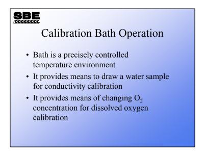
Baths of this design have been adapted for calibration of all of Sea-Bird's products. The basis is precisely controlled temperature and the ability to draw a water sample for salinity determination. The means to change partial pressures of Oxygen for SBE 43 calibration has been added.
