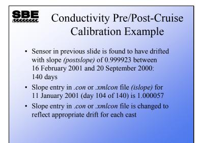
Refer to Application Note 31 for a detailed discussion of how to apply pre-/ post-cruise calibrations to SBE 4 conductivity sensors. Briefly, a calibration is done before and after the cruise. Let alpha be the conductivity that the instrument measured in the pre-cruise calibration, calculated using post-cruise coefficients. Let beta be the true conductivity of the pre-cruise calibrations. Then:
