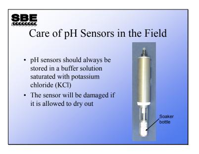
The pH electrode is porous and will dry out if left open to the air. It is always a good practice to keep it in clean, pH 4 buffer solution that has been saturated with potassium chloride (KCl). The electrolyte inside the pH sensor is saturated KCl.
