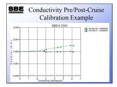
Conductivity sensors usually lose sensitivity as they drift. The drift takes the form of a slope. This is because the conductivity measured by the cell depends on the cell dimensions, which typically change due to fouling.
