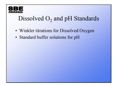
Dissolved oxygen sensors are calibrated in a bath that is plumbed with oxygen and nitrogen inputs. As gas concentrations are varied during calibration, Winkler samples are collected. These are titrated for dissolved oxygen concentration during the time of the calibration.
