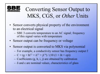
As we have discussed, a sensor has an active element that interacts with the environment, and a conditioning circuit that converts the reaction into a signal that is measurable with normal techniques (e.g., Analog/Digital conversion or counting of a frequency). Having acquired a digital representation of temperature or conductivity, we need to convert this into units useful to scientists and engineers.
