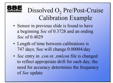
The factory oxygen sensor calibration sheet provides the value for *Soc* (that portion of the calibration sheet is not shown in the previous slide).
