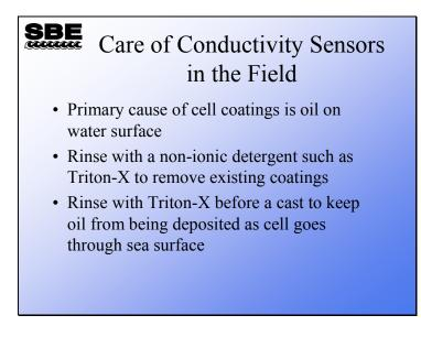
Sea-Bird supplies a small amount of Triton-X non-ionic detergent for cleaning conductivity cells. This will remove any oily coating, and an application before deployment will keep films from being deposited as the cell goes through the sea surface. Triton-X is a surfactant. A pre-deployment coating has the added advantage of wetting the electrodes, giving their surface a higher affinity to water.
