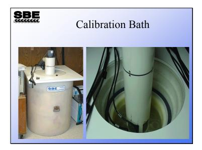
This bath design is common to all of Sea-Bird's calibration activities. The baths are highly insulated and well stirred, and they typically hold temperature to better than  $0.0005 \ ^{\circ}C$ .
