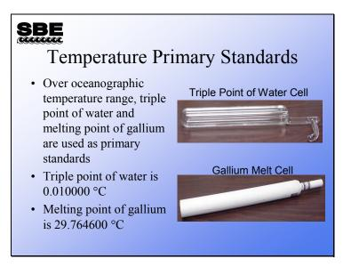
For calibration, one runs into the problem of knowing exactly what the temperature of a particular object is. If we only had thermometers to rely on, how do you know which one is right? Instead, we use physical standards. The Celsius temperature scale decrees that water freezes at 0 °C and boils at 100 °C; however, the freezing and boiling points are subject to uncertainties such as atmospheric pressure. So, instead of the freezing and boiling points, we use two other points:
