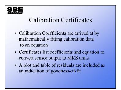
The calibration certificate is a listing of all the information required to convert sensor output to scientific units. There is also a table of calibration data and a plot of residuals that indicates a goodness-of-fit. Residuals are expressed as the difference between the instrument parameter and the bath parameter (the *true* value):
