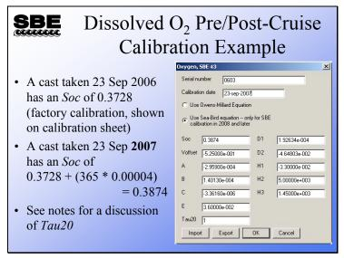
*A word about Tau*: Tau, a term in the Sea-Bird equation, relates the change in oxygen sensor voltage to dissolved oxygen concentration.
