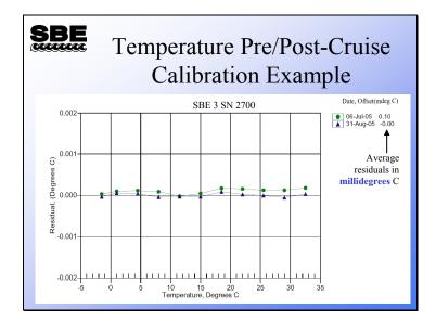
The average residuals (residual = instrument temperature – true temperature) are shown to the right of the plot.
