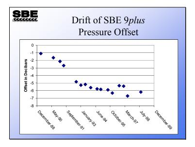
This sensor shows a typical drift until October 1995, when it begins to change in a more random manner. The random behavior indicates that it is time for a calibration and test by the factory.
