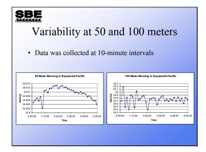
This slide shows data from a mooring near the equator. The 50-meter mooring data shows a change in salinity that might be from tidal influence. The change observed here is of similar magnitude to the correction that might be applied to CTD data based on the difference between discrete samples and the CTD.
