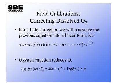
Our goal is to rearrange the equation into a linear form that we can use in a linear regression of Winkler titration dissolved oxygen versus SBE 43 voltage output. To simplify this we will collect terms and express oxygen saturation and the corrections for pressure and temperature as *phi*.
