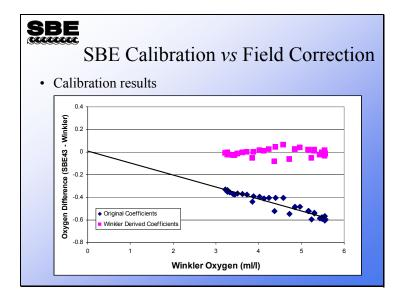
This plot shows the improvement in agreement between the Winkler titrations of dissolved oxygen and the SBE 43 measurement of dissolved oxygen after application of the Winkler-derived *Soc* and *Voffset*. The blue diamonds are the difference between the Winkler values and the SBE 43 values using *Soc* and *Voffset* from the most recent calibration. The pink squares are the difference between the Winkler values and the SBE 43 values using *Soc* and *Voffset*.
