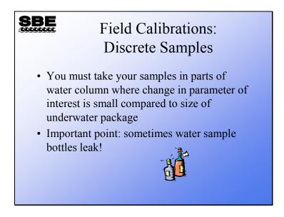
Most instrument packages are more than a meter tall. If you take your samples for field calibrations in a part of the water column where the salinity or oxygen concentration is changing rapidly, you will not get a good sample for calibrating. Not only is there mixing of the water inside the water sampler, but you will be comparing a large mixed sample with a virtual point sample from the sensors.
