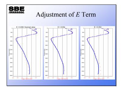
We can make the adjustment to *E* empirically. The plots above show the discrepancy between the SBE 43 calculated oxygen and the Winkler titrations with a series of *E* values. Clearly, the middle value of E = 0.034 gives the best agreement.
