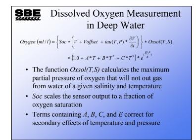
Recall the dissolved oxygen equation; basically it is a scaling of oxygen saturation based on sensor output with a correction for temperature sensitivity and for pressure sensitivity. In the following discussion we will explore the pressure correction coefficient and learn how to fine tune it with adjustments to E.
