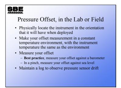
This discussion is primarily intended as a guide for the SBE 9*plus* with a Digiquartz pressure sensor. However, the technique is sound for all pressure sensor types regardless of sensitivity.
