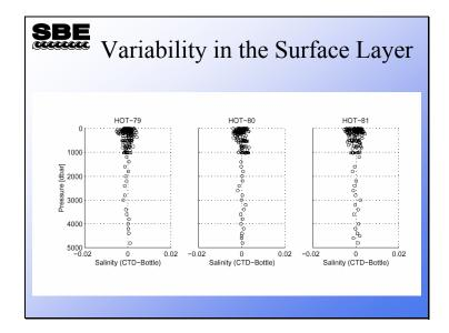
These data are taken from 3 cruises off Hawaii. The problem with using the surface layer to correct CTD conductivity is obvious.
