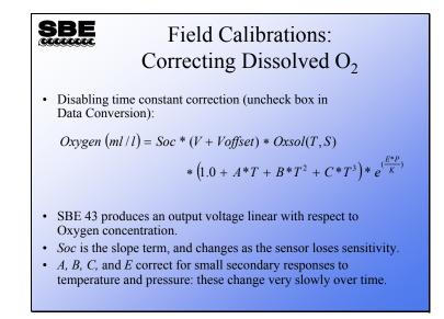
The SBE 43 is expected to provide an output voltage that is linear with respect to oxygen concentration.
