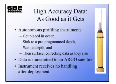
These CTDs have a significant advantage over the usual deployments with regard to conductivity drift. They are deployed from ships with their conductivity cells full of de-ionized water, and have no contact with ships or humans for the remainder of their lives. They are never exposed to the sea surface near a ship with its oil film. Finally, their cells are never allowed to dry, so the electrodes are always stored in biology-resistant water.
