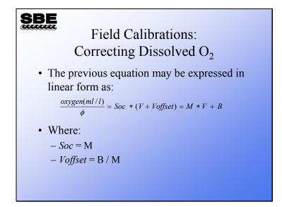
Finally, Winkler titration values divided by *phi* is the independent variable and SBE 43 output voltage is the dependent variable. Note that *Soc* and *Voffset* are constants, so the right side of the equation is expressed as a slope (*Soc*) multiplied by a variable voltage plus a constant offset (*Voffset*).
