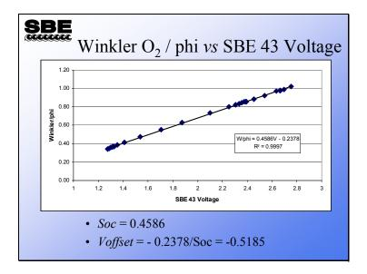
Here is a plot and regression of some data gathered in Puget Sound. Even though Puget Sound is not a well-mixed environment, there is a very strong relationship between Winkler  $O_2 / phi$  and SBE 43 Voltage.
