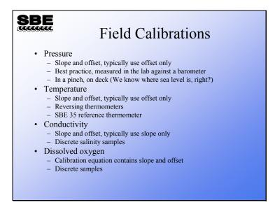
The configuration (*.con* or *.xmlcon*) file has entries for *slope* and *offset* for all standard sensor types except dissolved oxygen. These entries are the means to make adjustments in the sensor calibration by using field observations.
