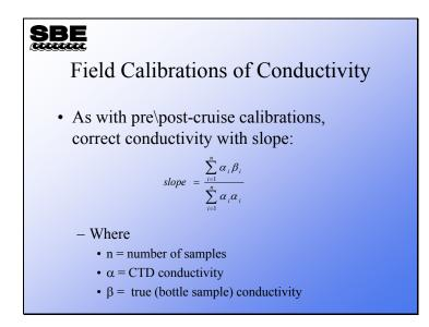
The summation symbol, Sigma ( $\Sigma$ ), denotes the addition of a series of values. The script on the bottom of the  $\Sigma$  is the index of the starting value, the script on the top is the ending value. We wish to use all suitable samples so we will start with one and end with n, the total number of samples.
