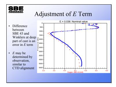
As you might imagine, the term in the equation that corrects for pressure effects has little effect in the upper part of the profile. The slide above illustrates that as the pressure increases, the response of the instrument deviates from the Winkler titrations. We can improve the agreement of the SBE 43 and the Winkler titrations by adjusting E.
