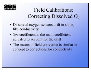
Terms that can be modified by the user to adjust the calibration of the SBE 43:
