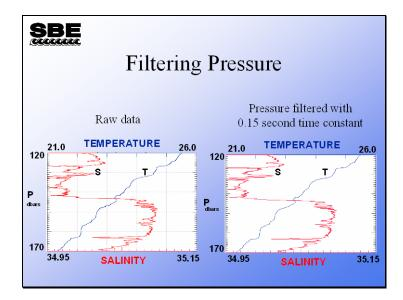
The left plot shows some *dithering* in the data that is eliminated by filtering the pressure.
