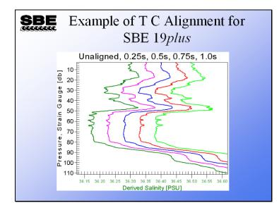
This is from the extra credit data set. The left most trace is the original unaligned data and the others, from left to right, are aligned from 1 to 4 scans. The optimal alignment value may lie between 0.25 and 0.5 seconds; it is left for the reader to experiment and find it.
