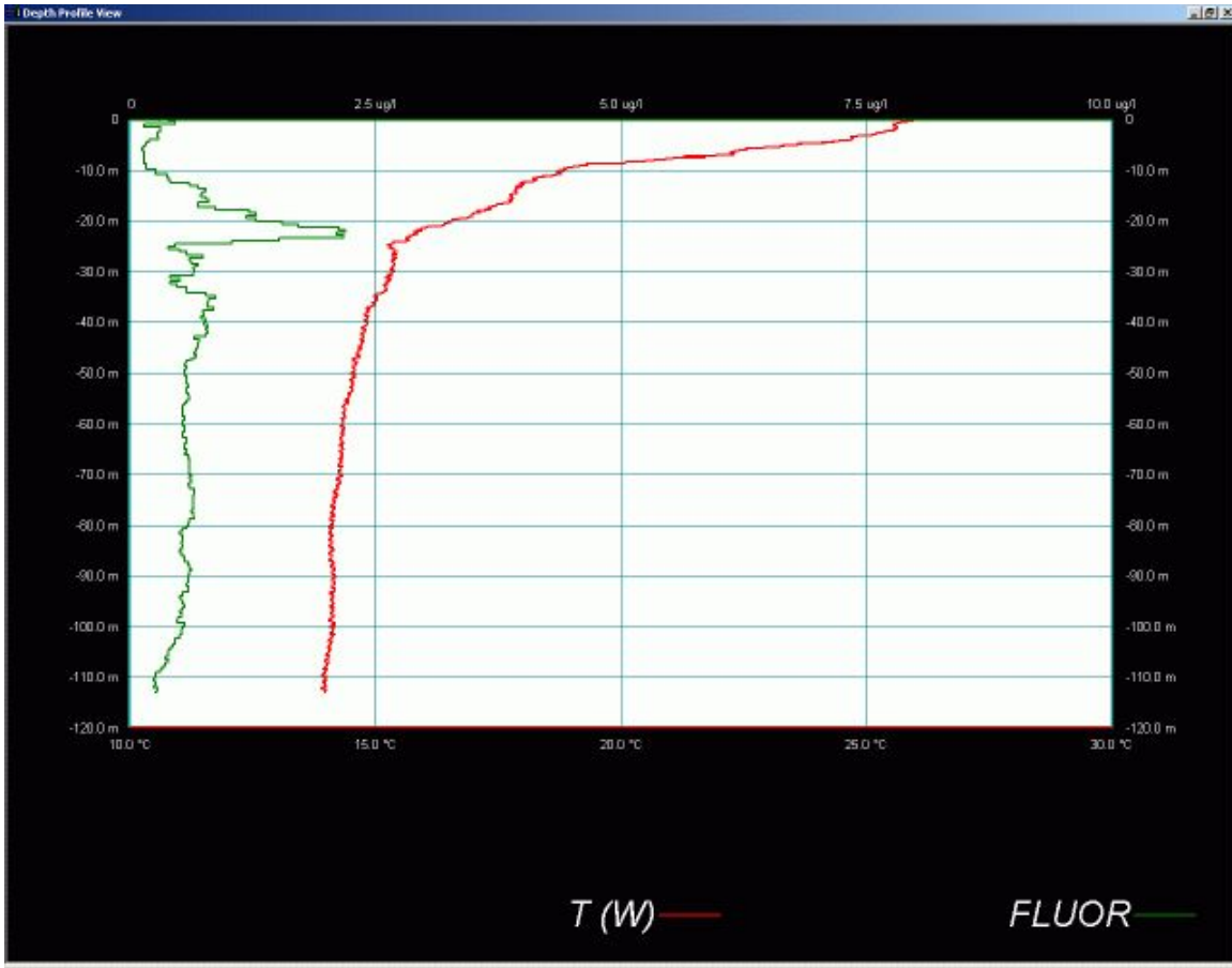
Figure A-6: SatView plot demonstrating Integrated Fluorometer
