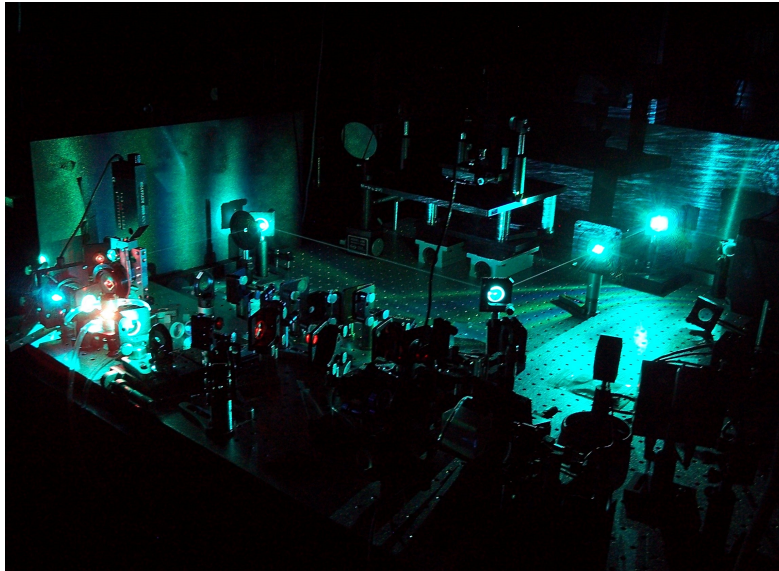
Figure 1: SIRCUS Ti:Sapphire laser pumped with a 25W Argon Ion Laser at NIST
