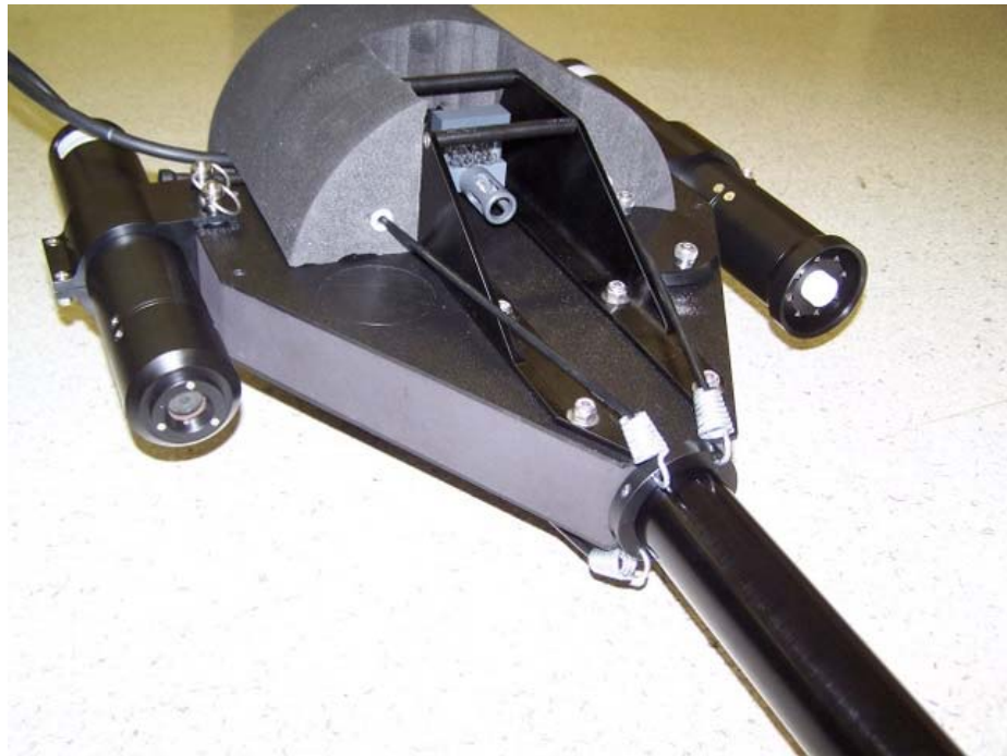
Figure D-6: Float installation for Profiler II Surface Mode
