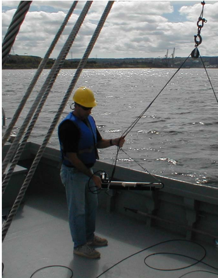
Figure D-3: Frame Mounted Deployment
