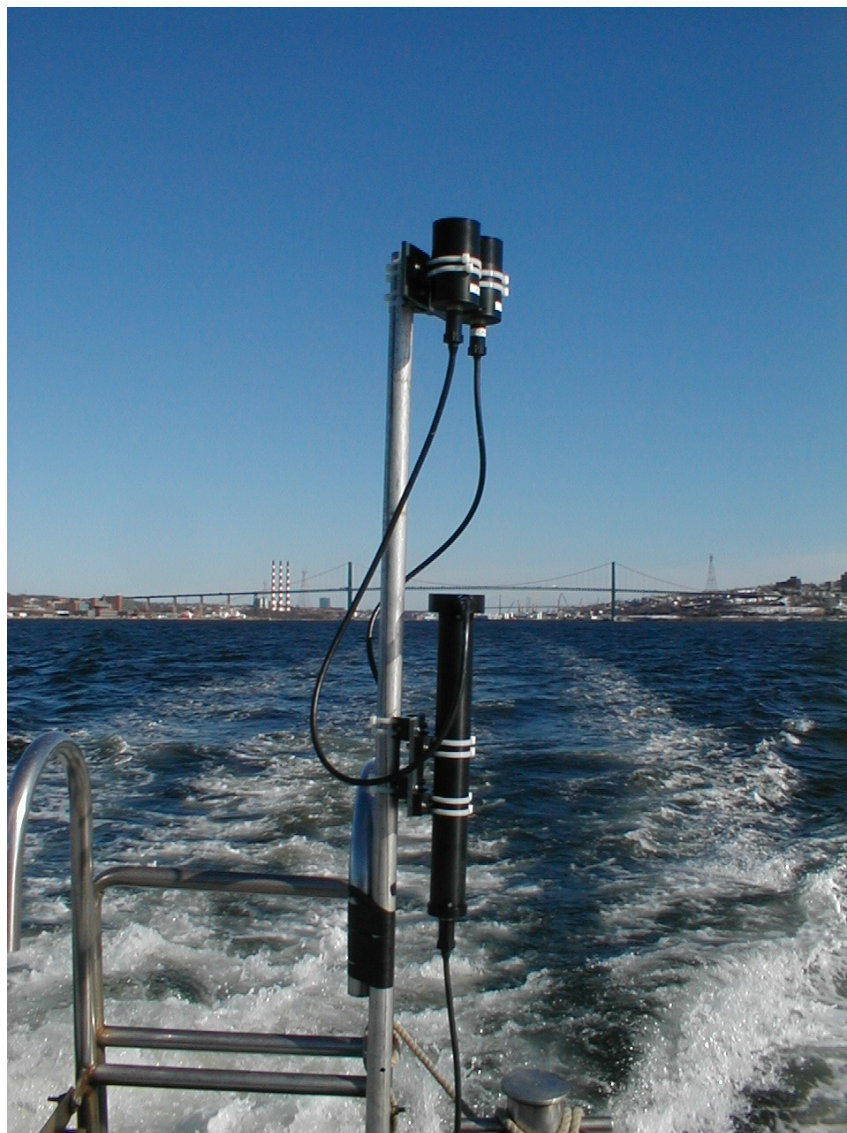
Figure A-10: A Surface Reference System Field Test
