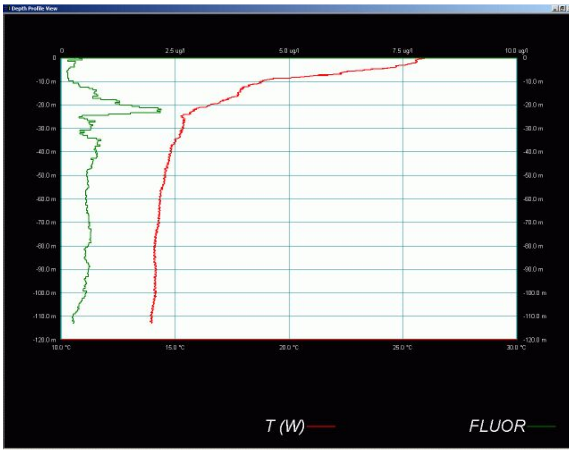
Figure A-6: SatView plot demonstrating Integrated Fluorometer
