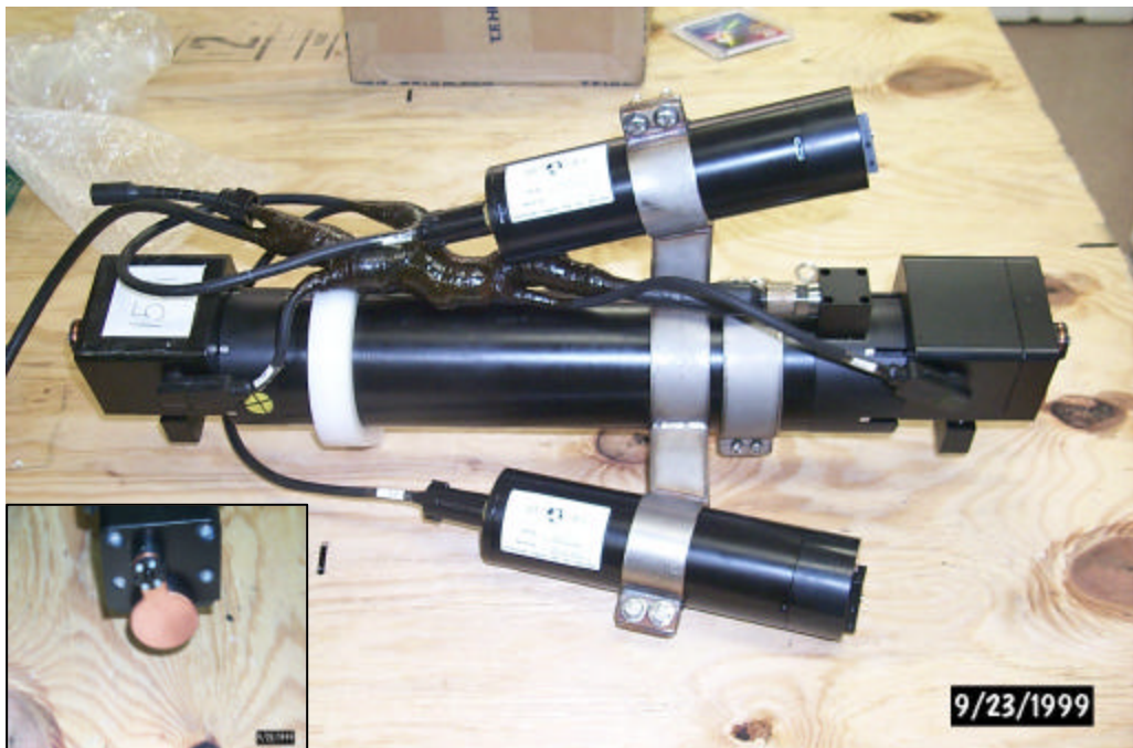
Fig. 2. (a) Example of water-leaving radiance spectra derived from radiometric measurements collected at the LEO-15 site (25 km offshore, 24 m water depth). (b) Photograph of an optical system used to measure inherent and apparent optical properties: upwelling radiance and downwelling irradiance, chlorophyll fluorescence, and the volume scattering function. Insert photograph shows a special copper shutter device for minimizing biofouling of the sensors. Photographs provided by Derek Manov.
