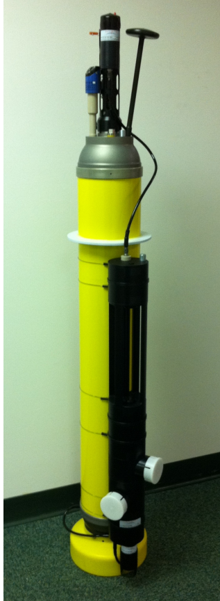
Figure 1: Biogeochemical float with optics suite attached to side and irradiance sensor, CTD, Optode, and antenna on top.
