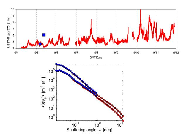
Figure 1. Beam attenuation coefficient is an indicator of changes in particle concentration near the seabed (top panel). The blue symbols denote sample times of the VSF measurements shown in the bottom panel. The red and blue symbols in the bottom panel represent VSF data from the LISST-100 Type B and LISST Floc instruments, respectively, and the black lines denote the "merged" VSF estimated from the adjusted LISST Floc data.
