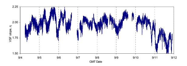
Figure 2. Slope of the near-forward VSF based on the power law fit  $\beta(\psi) = \beta_0 \psi^{-\eta}$ , which indicates changes in the particle size distribution of suspended particles.
