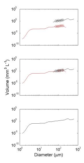
Figure 3. Example of the LISST-100 Type B and DFC size distributions during adjustment that results in a merged size distribution 1.25 µm – 1 cm in diameter. The red line represents the LISST-100 Type B size distribution and black line represents the DFC size distribution. The circles mark the region of overlap used for adjusting both size distributions. The adjustment factor for this data was 212. The data was collected on September 4, 2005, at 0444 GMT.
